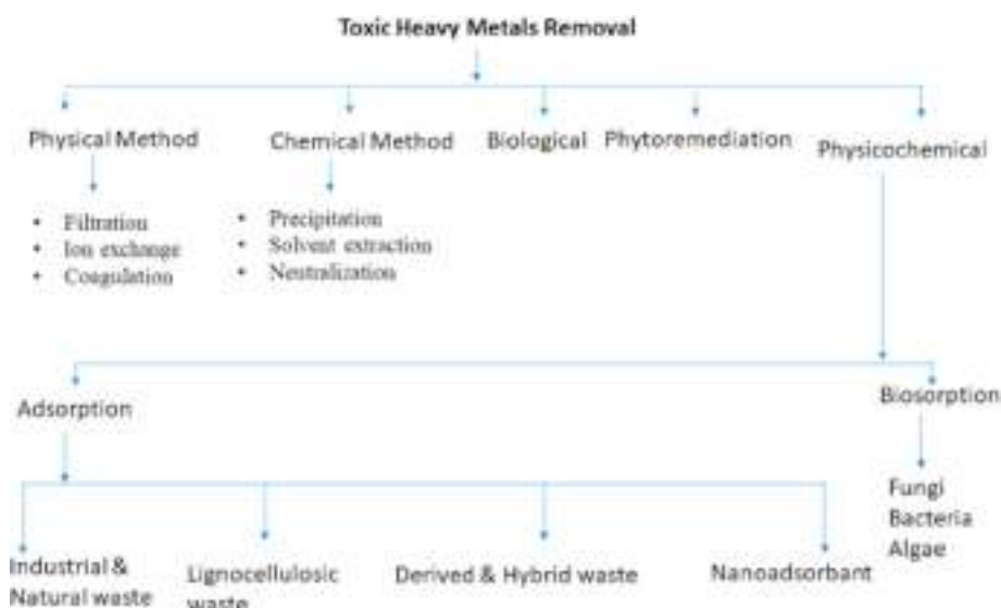
Fig. 1. Scheme of various methods involved in heavy metal remediation with special emphasis on bio-sorption and adsorption.
