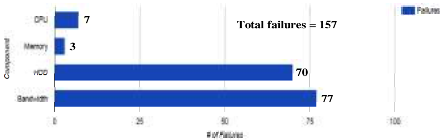
Figure 11 Component failures by resource type for the initial test-case CCS (144 VMs) simulation as shown in Table 3 (see online version for colours)
