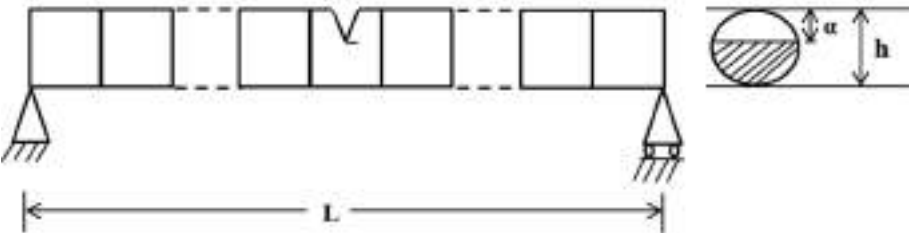
Fig. 2. Discretized model of a beam with an open crack.
