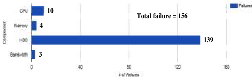
Figure 3 Component failures by resource type for the first test-case CCS (144 VMs) as shown in Table 3 and simulated over ReliaCloud-NS (see online version for colours)
