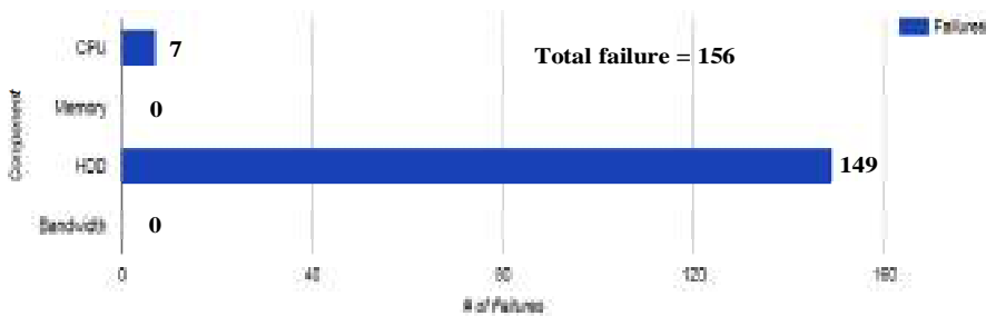
Figure 5 Component failures by resource type for the second test-case CCS (236 VMs) as shown in Table 4 and simulated over ReliaCloud-NS (see online version for colours)
