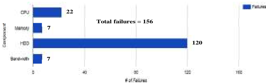
Figure 9 Component failures by resource type for the initial test-case CCS (236 VMs) as shown in Table 4 (see online version for colours)
